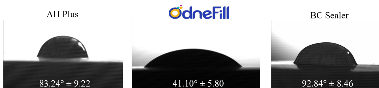
Figure 1: Wettability comparison between AH Plus®, Odne™Fill and BC Sealer.
